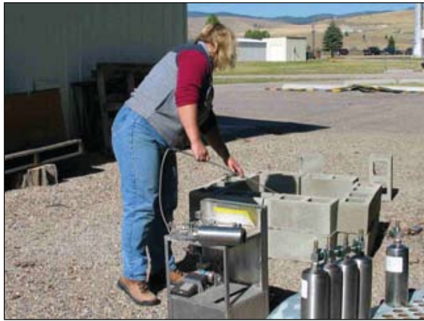
LEFT: Sherry Dingle, a fire lab employee, conducts a controlled test using commonly burned items to determine the amount of toxic substances released in a campfire.
